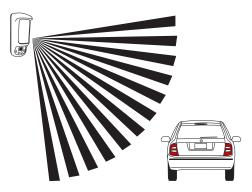
In order to maximize detection efficiency, choose a location that is most likely to intercept intruders moving across the coverage area at a 45 degree angle.
